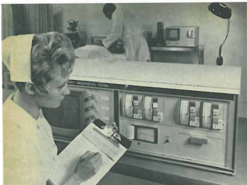
Fig. 1. Patient monitoring system gives doctor on-the-spot data and allows one nurse to monitor up to eight patients.
