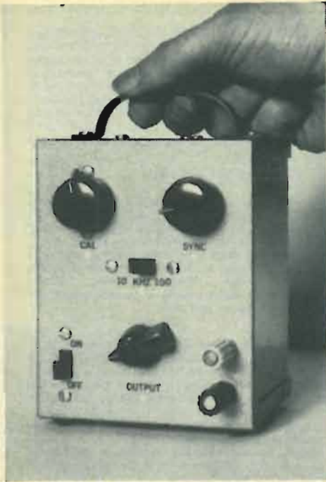
Fig. 1. Front view of the portable dual-range IC frequency standard showing the controls used in calibrating the instrument for 10- and 100-kHz signals.
