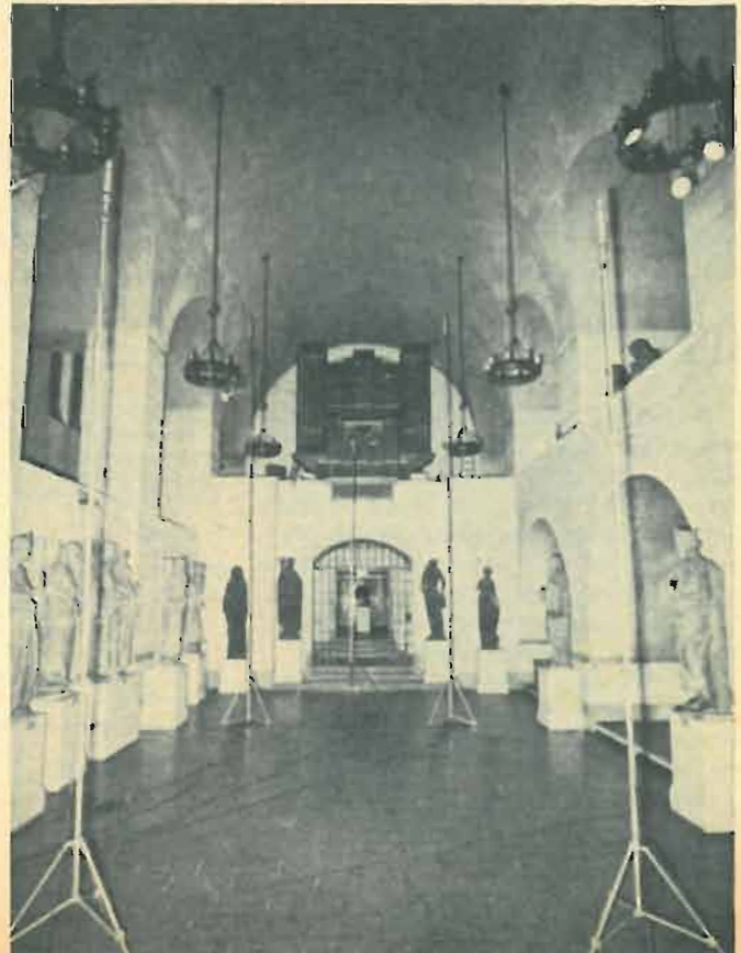
Microphone setup in Busch-Reisinger Museum at Harvard during Columbia recording of organ music performed by E. Power Biggs. Five microphones were used; front center information from fifth mike was mixed into front left and right.
